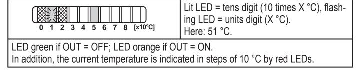
▶ Press ▶ or ✓ as often as required. Each press of the pushbutton shifts the flashing LED (units digit) by one position in the indicated direction.
