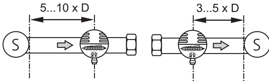
D = pipe diameter; S = sources of interference
