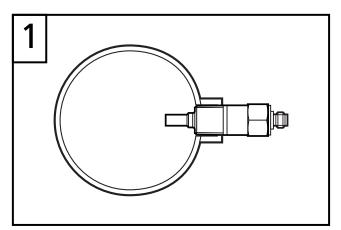
To avoid malfunction a minimum distance between the flow monitor and bends, valves, changes in cross-section or such like must be observed:
