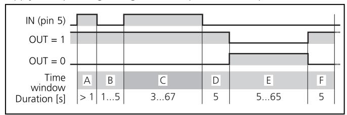
Within the time windows A, B, C the output is switched depending on the flow: output closed (OUT = 1) if flow  $\geq$  SP / output open (OUT = 0) if flow < SP.
