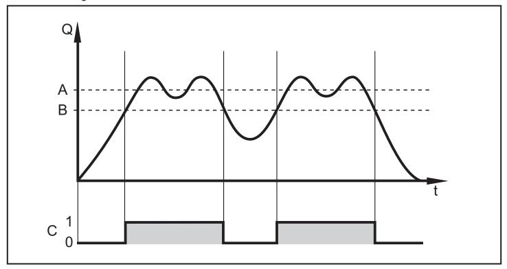
A = requested flow; B = switch point; C = switching output
