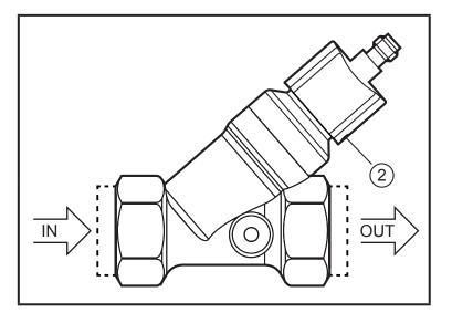
► Insert the unit into the pipe according to the direction of flow (arrow) and tighten.
