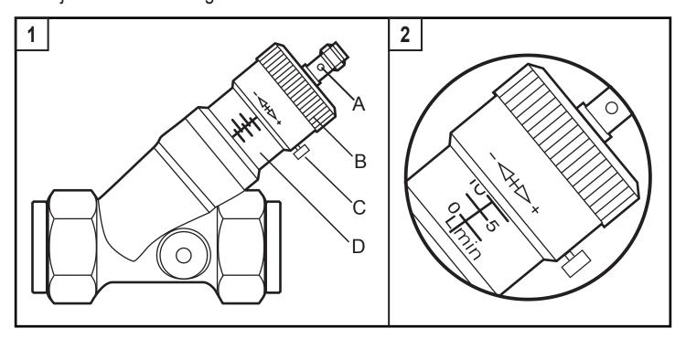
A: LED; B: setting screw; C: lock screw; D: setting scale
