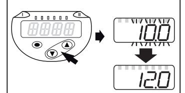
Numerical values are incremented continuously with [▲] or decremented with [▼].
