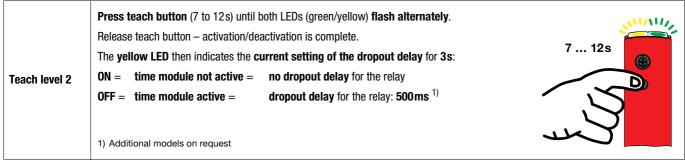
Dropout delay: if the object is no longer present, the output switches with a time delay.
