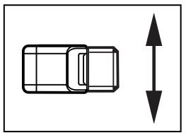
The objects to be detected are to move transversally to the lens of the sensor. In case of other directions of movement it should be tested before whether the switching function is guaranteed.
