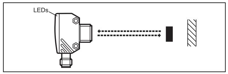
➤ Align the diffuse reflection sensor to the object to be detected and secure it to a bracket..
