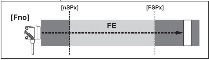
[nSPx] = switch point "near"; [FSPx] = switch point "far"; FE = window
