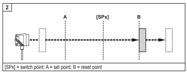
When the output function [Hnc] was selected, set and reset point are reversed. The output is switched off when the object approaches. When the object is removed, the output switches on.
