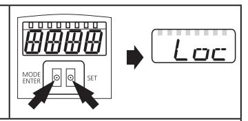
[Loc] is displayed briefly if you try to change parameter values on the locked unit during operation.
