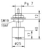
Details of float location 17 mm for density1 g/cm<sup>3</sup>. The device is delivered without a seal.
