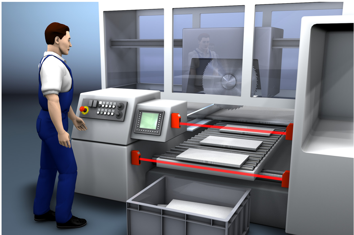
Figure 5.2: Access guarding / intervention control on sawing machines
