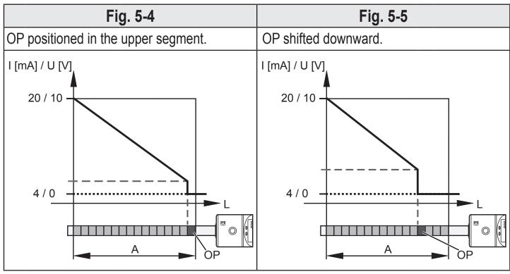
A: Active zone OP: Measuring segment overflow prevention OP L: Level
