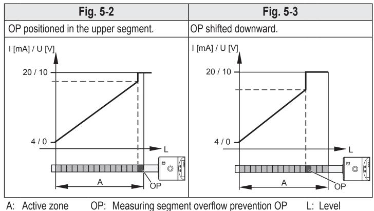
The measuring range is limited by the active measuring segment OP. If the level reaches the measuring segment OP, the output signal jumps to its maximum value (20 mA / 10 V).
