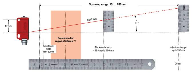
1) The ability of the sensor to reliably detect reflective surfaces or transparent objects is the strongest in the recommended working range. The sensor can also reliably detect such objects in the entire scanning range; however, the performance reserve is reduced in comparison to the recommended working range.
