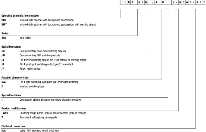
N/A cable, PVC, standard length 2000 mm S12 M12 connector, 4-pin, axial
