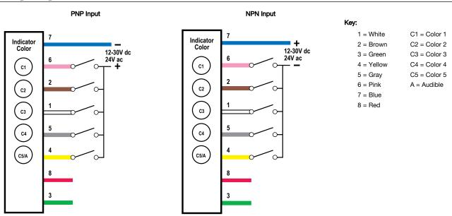
Pin 4 could activate the corresponding color or the audible function, if available. Pins 3 and 8 are not used.
