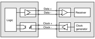
Rotary encoder Interface electronics
