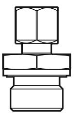
The progressive ring fitting consists of the three parts screw fitting (A), cutting ring (B) and coupling nut (C).
