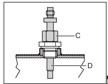
4. Tighten the coupling nut manually and mark its position with a line (E).
