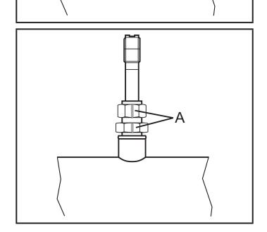
Tighten the coupling nut with a tool by 1¼ turn (tightening torque 45 Nm).
