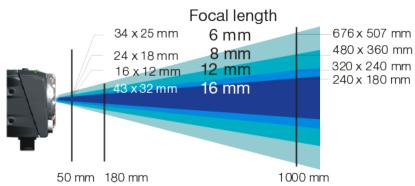
Fig. 16-4 Field of view for sensor models
