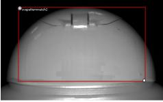
Fig. 8-3a Pattern detection of a shampoo bottle seal:  $\ensuremath{\mathsf{OK}}$
