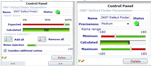
Fig 8-11: Control panel 360° Defect finder, page 1 and 2
