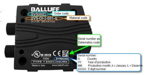
Fig. 16-1 Sensor type identification
