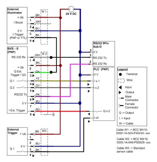
Fig. 3-7: Wiring diagram of the BVS-E sensor ID and UR
