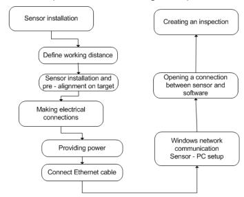
Fig. 3-2: Initial startup sequence
