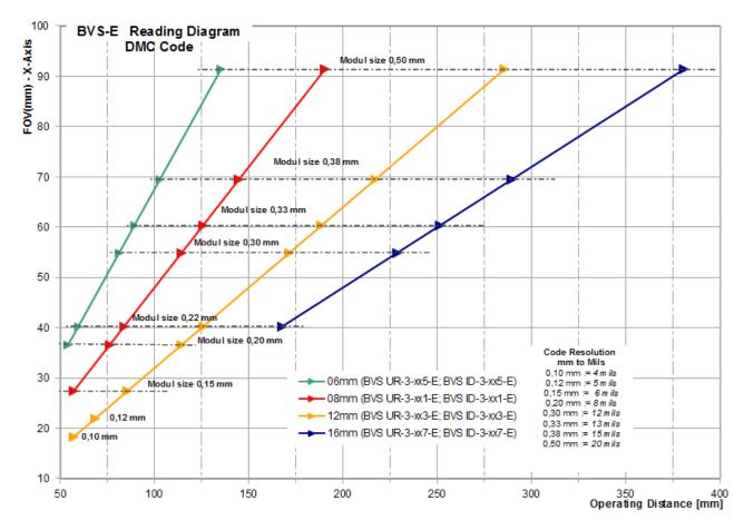
Fig. 16-7 Read field diagram for a Data Matrix code Minimum distance of BVS yy-3-0x7-E: 180mm Minimum distance of BVS yy-3-1x7-E: 230mm
