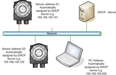
Fig. 4-3: DHCP connection of the sensor
