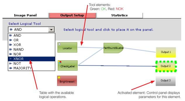
Fig. 10-1: "Set outputs" view with tools and logical operations
