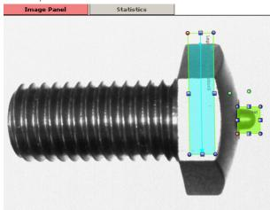
Now enlarge the ROI of the tool - the position change of the part must always take place within the ROI, otherwise the position cannot be located. Now adjust the permissible Maximum to your application.
