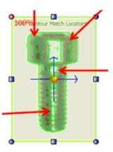
2.) Removing weak reflection contours using the Noise Suppression parameter. Contours with weak contrast or short length are removed by adjusting the Noise Suppression parameter.
