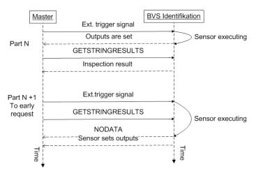
Fig. 9-2: Synchronous communication
