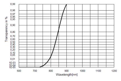
Fig. 16-3: Filter diagram of infrared models
