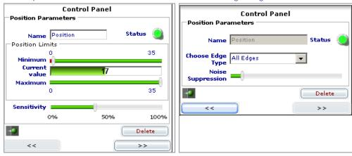
Fig.8-10: Control panel for "Check Position", page 1 and page 2
