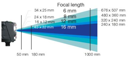
Fig. 16-5 Field of view for sensor models
