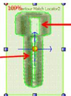
Be sure when changing the Noise Suppression parameter you do not remove any contours important for the inspection, e.g. on the screw
