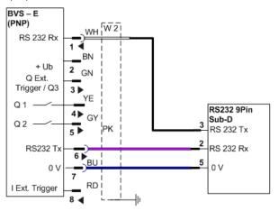
Fig. 9-1: Wiring the RS232 interface to a Sub-D 9-pin connector
