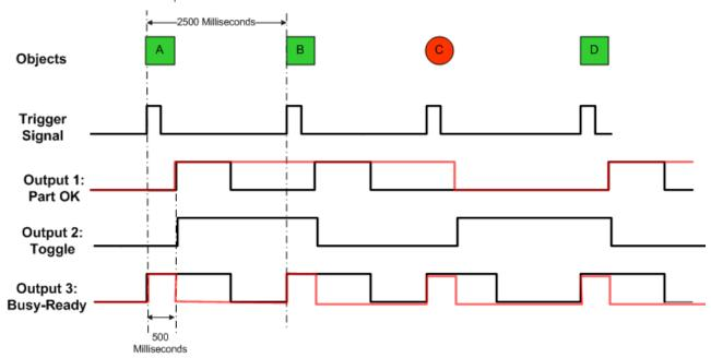
Fig. 10-3: Diagram for output timing
