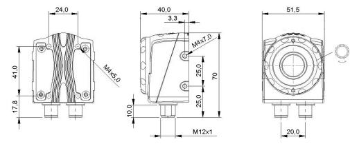
Fig. 16-2: BVS-E, dimensions (in mm)
