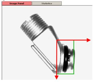
The figure above illustrates this using the example of the "Pattern detect" locator. If the locator finds the taught feature in the reference image, it changes the position of its ROI in the image, and the determined position is then the upper left corner of the ROI. All other tools are oriented by this POSITION.
