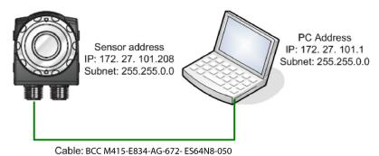
Fig. 3-8: Direct connection of the sensor
