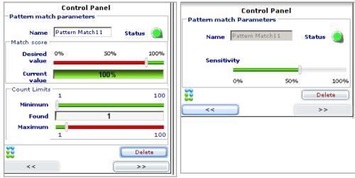
Fig.8-9: Control panel for "Pattern detect", page 1 and page 2
