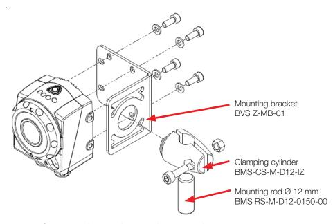
Fig. 3-3: Sensor attachment using mounting accessories Select the mounting location of the sensor so that the inspection object is not subjected to direct sunlight or strong ambient light (room lighting, optical sensors, lasers) while it is in the sensor field of view.
