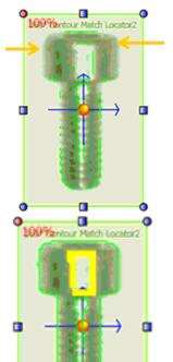
3.) Use the mouse to remove other unimportant contours. Placing the mouse pointer over a selected or deselected contour will show it in yellow.
