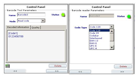
Fig 8-14: Control panel for Read Barcode, page 1 and page 2  $\,$
