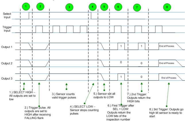
Fig.11-1: Timing diagrams Phase 1 to 8
