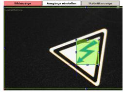
The target pattern is the lightning bolt - defined by the ROI. Also displayed is the orientation of the pattern - represented by the dark blue coordinate system. The zero point always lies on the VERTICAL AXIS!
