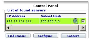
The control panel shows all the sensors found using the "Find sensors" function. The following information is displayed for each sensor:
