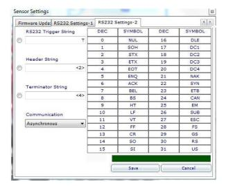
The replies to the GETSTRINGRESULTS command differ essentially from the other commands. For result transmission the BVS-E Identification sensor has two different operating modes: Synchronous and asynchronous communication.
