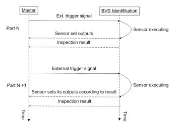
Fig. 9-3: Asynchronous communication
