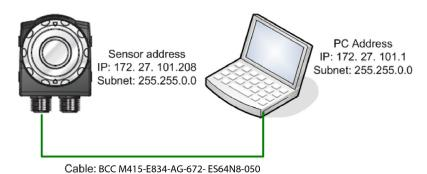
Fig. 4-2: Direct connection of the sensor
