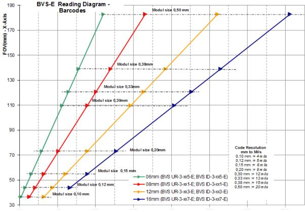
Fig. 16-6 Read field diagram for a barcode
