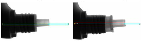
Fig. 8-4a Position checking of the spout of a dish liquid bottle:  $\ensuremath{\mathsf{OK}}$
