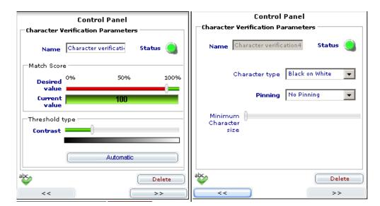
Fig 8.13: Control panel "Optical character verification" Page 1 and Page 2 The OCV tool includes the following parameters:
