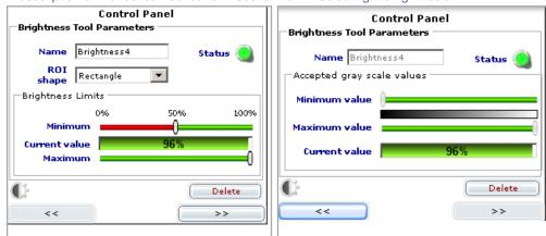
Fig.8-6: Control panel for Brightness, page 1 and page 1
