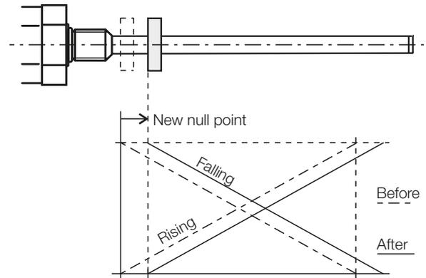
Fig. 6-2: Reading new null point (offset shift)
