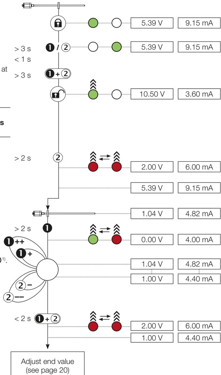
1) Briefly press button: Current value is increased or decreased by approx. 1 mV or 1 µA. If a button is held down longer than 1 s, the step interval is increased.
