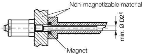
¹) Min. Ø D2 = Minimum diameter of the bore (see Tab. 4-1)
