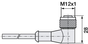
Fig. 12-7: Connector type BKS-S116-PU-\_\_
