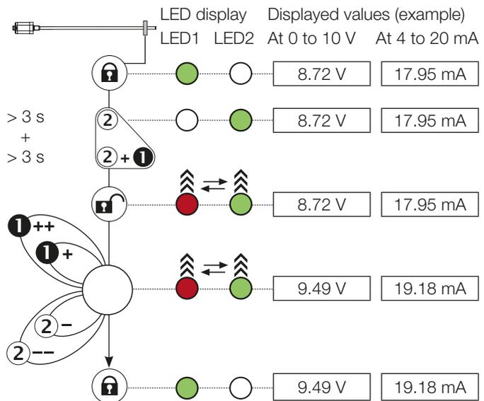
1) Briefly press button: Current value is increased or decreased by approx. 1 mV or 1 µA. If a button is held down longer than 1 s, the step interval is increased.
