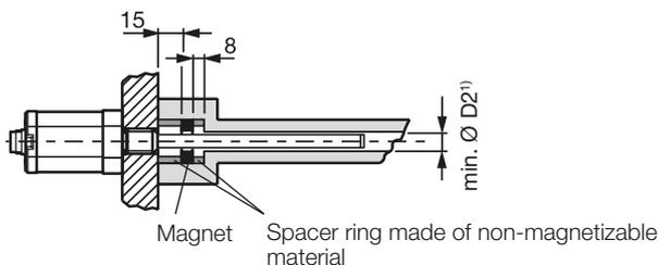
¹) Min. Ø D2 = Minimum diameter of the bore (see Tab. 4-1)
