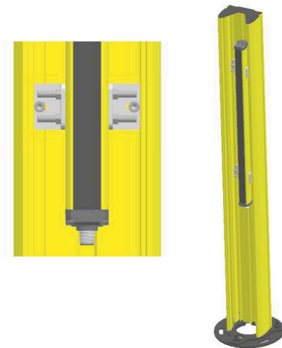
Figure 21: Installation – height adjustment
