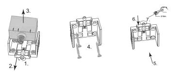
1. Loosen the central screw under the sensor connection.
